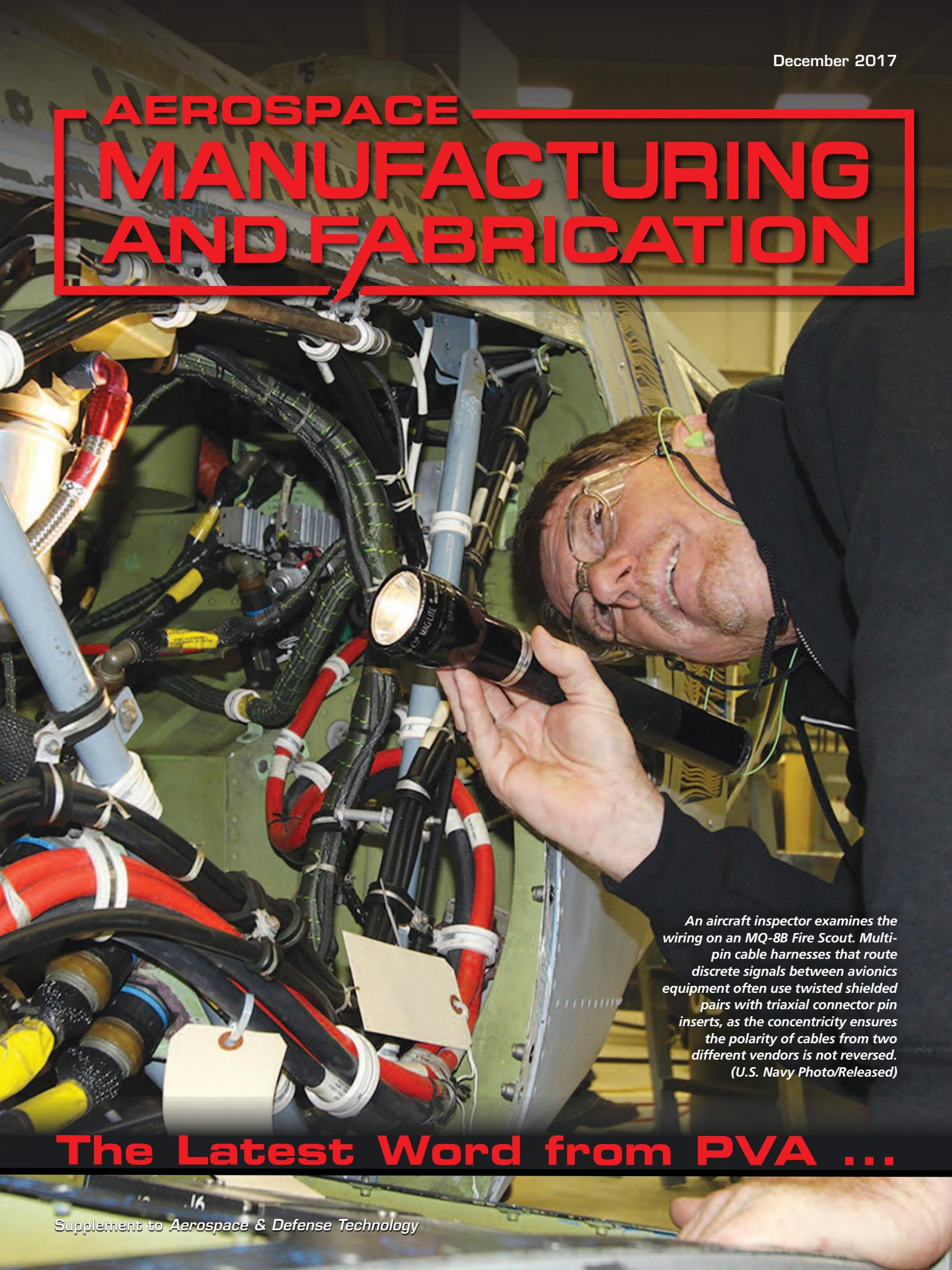
*An aircraft inspector examines the wiring on an MQ-8B Fire Scout. Multi-pin cable harnesses that route discrete signals between avionics equipment often use twisted shielded pairs with triaxial connector pin inserts, as the concentricity ensures the polarity of cables from two different vendors is not reversed. (U.S. Navy Photo/Released)*
