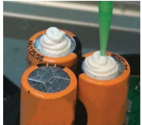
Dispensing TIM onto a capacitor
