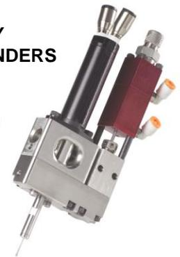
With the use of centrifugal force to transfer the silicone lubricant to the inside walls of the syringe, there is no longer a burst of atomizing air into the syringe. This dramatically reduces the amount of silicone mist that gets generated and sent into the air around the coating station to maintain a much cleaner process area.
