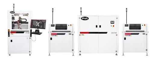
**Coat + IR UV** Delta 8 + Queue Inspection Conveyor + DeltaTherm + Queue Inspection Conveyor
