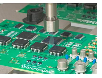
**Conformal coating** is a protective coating or polymer film that "conforms" to the circuit board's inherent irregularities to protect electronic circuits from harsh environments. Conformal coatings are a breathable protective layer that protects a printed circuit assembly from its exposed environment by filtering out airborne contaminants and maintaining longterm surface insulation resistance. Entrapped moisture, however, is allowed to escape.
