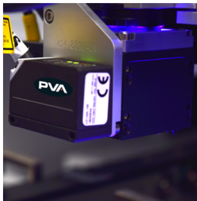
PVA-SMT-LHS laser height sensor
