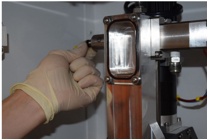
Figure 6: Disconnect Power Transducer Cable
