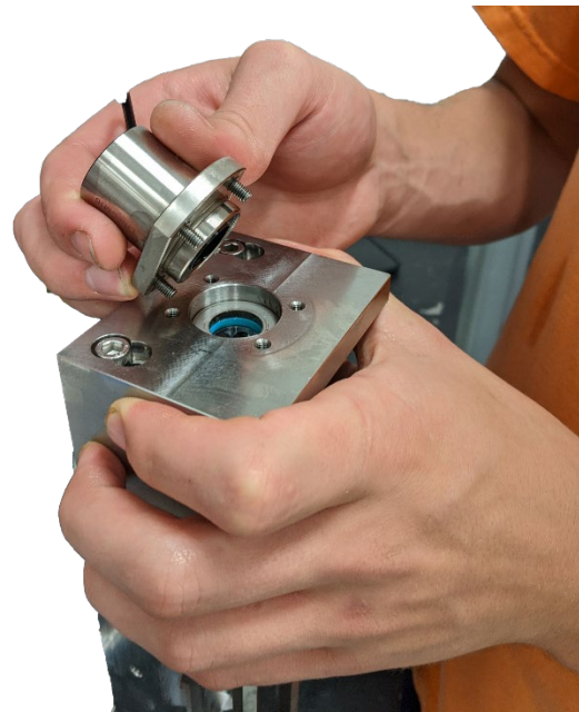
Figure 28: Remove Linear Bearing
