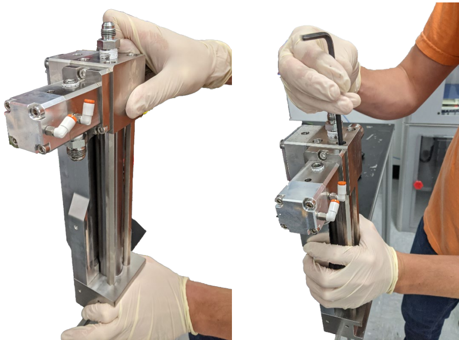
Figure 35: Install Upper Manifold Block
