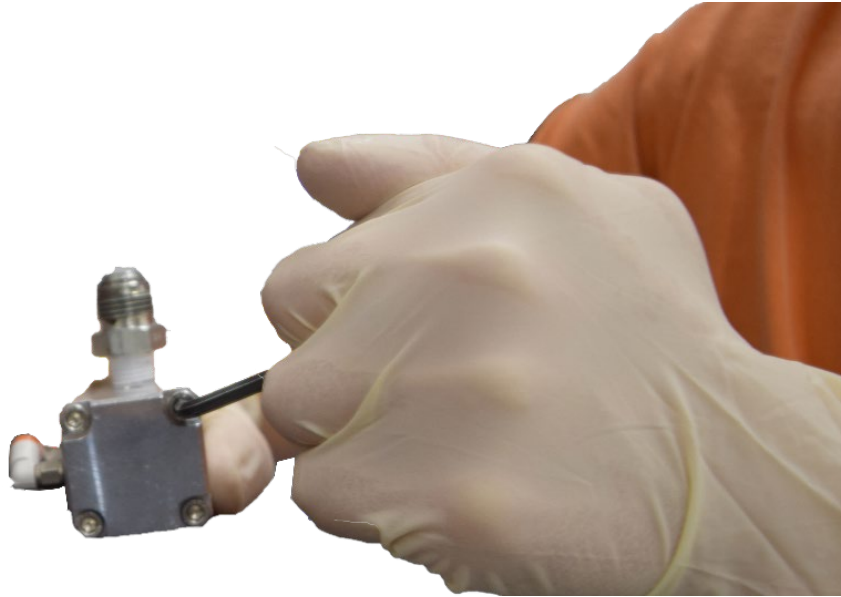
Figure 23: Remove Air Cap
