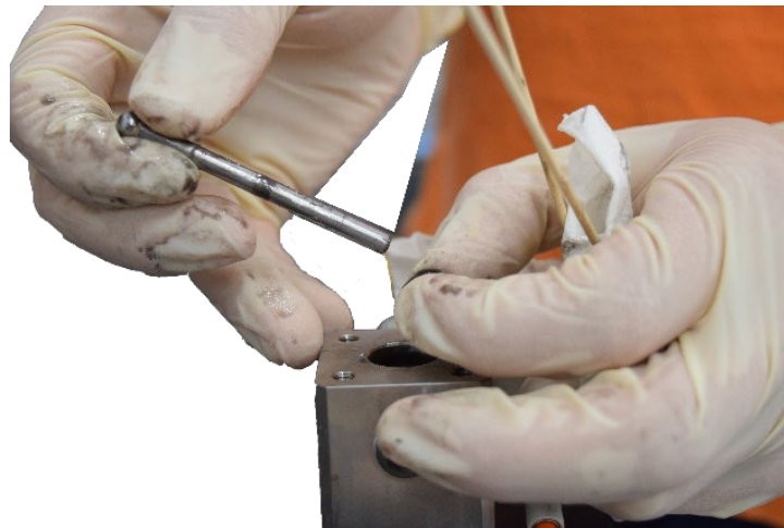
Figure 26: Remove Rod and Clean
