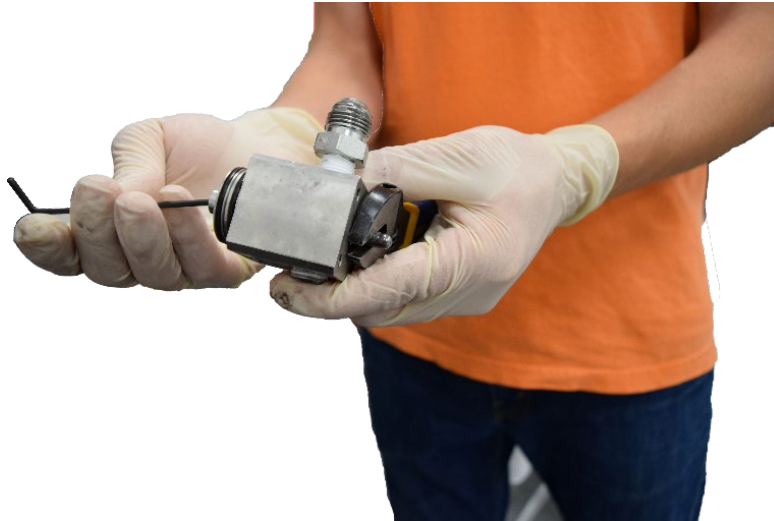
Figure 25: Remove Air Cap Entry Screw
