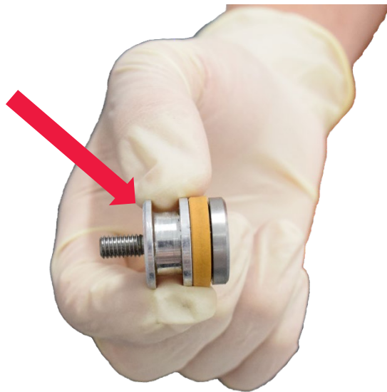
Figure 18: Install Wear Ring Groove
