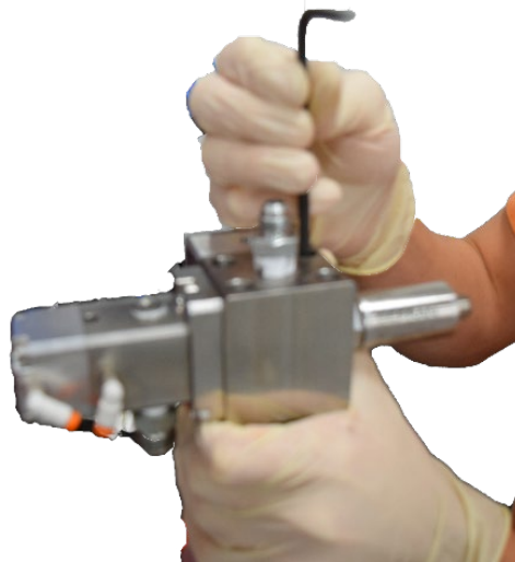
Figure 12: Remove Screws from Upper Manifold Block
