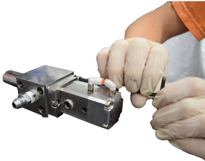
Figure 20: Remove M5 Socket Head Cap Screws
