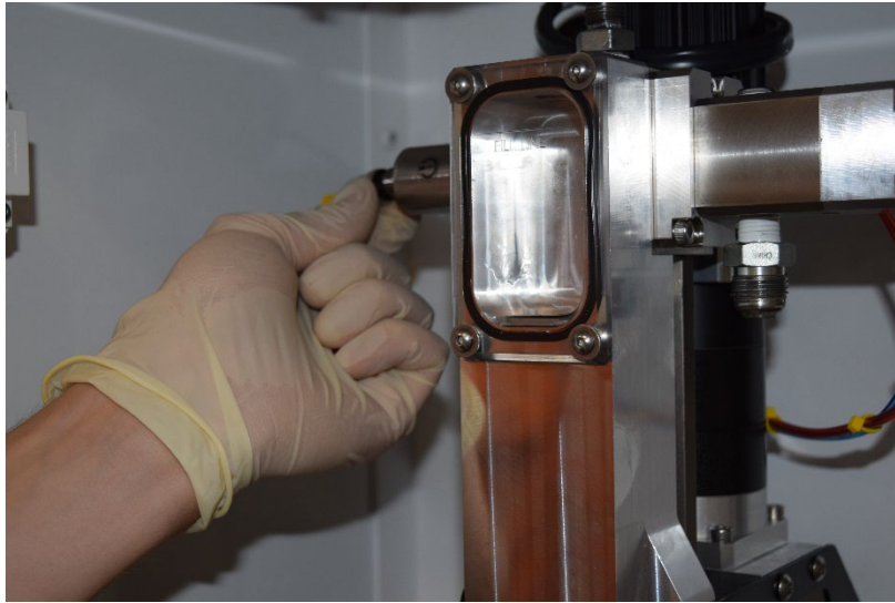
Figure 40: Reconnect Power Transducer Cable
