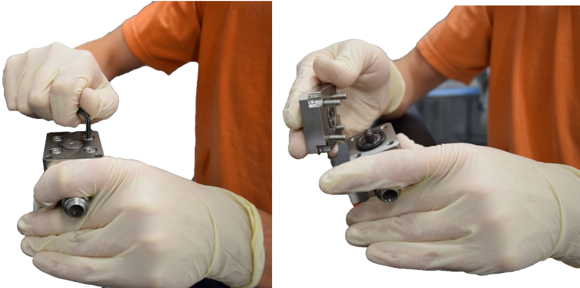
Figure 21: Remove Screws and Seal Plate
