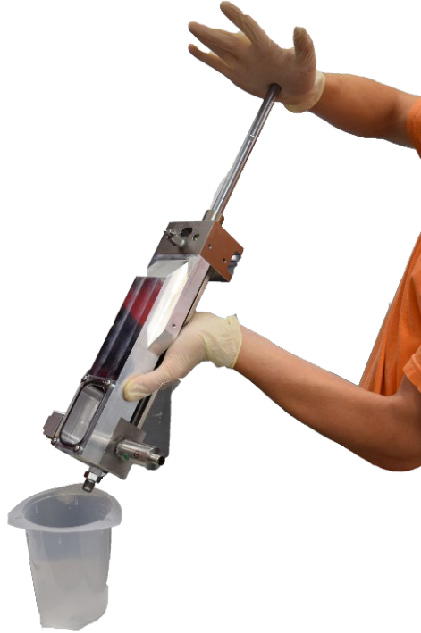
Figure 11: Push Rod to Discard Material
