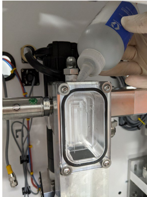
Figure 38: Add Material to Fill Line
