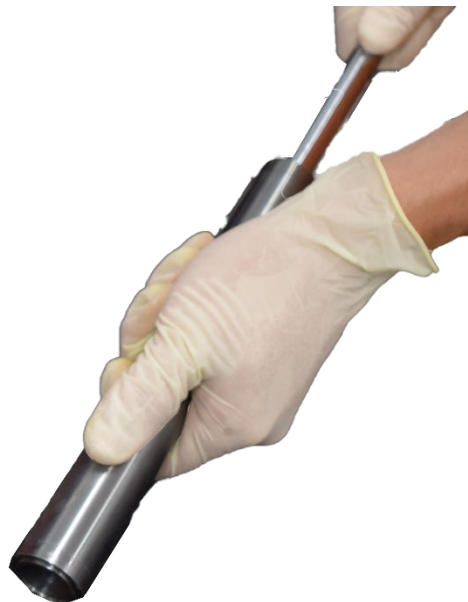
Figure 14: Remove Piston from Sleeve
