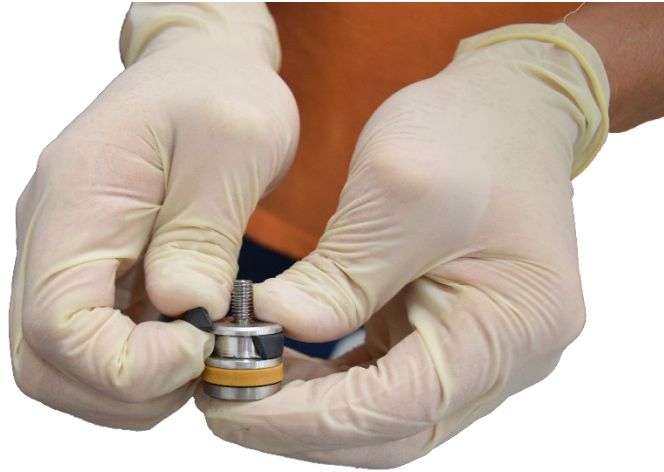
Figure 19: Install Wear Ring
