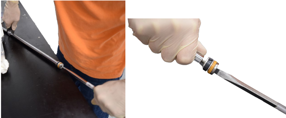
Figure 15: Remove Lip Seal Screw
