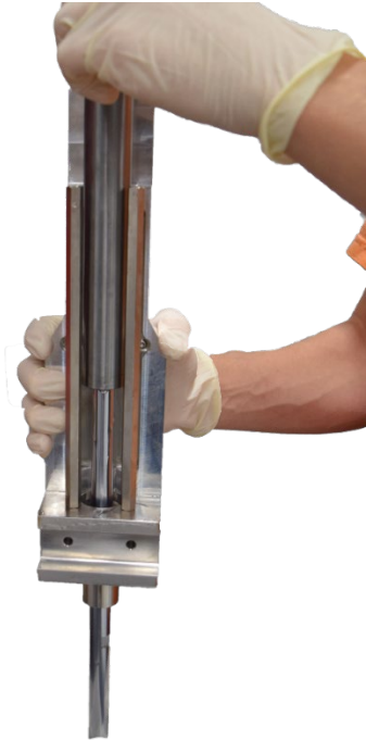
Figure 13: Separate Sleeve Rod Assembly
