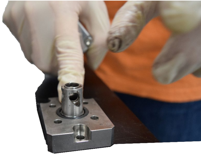
Figure 27: Install Seal Spacer
