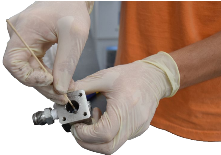
Figure 22: Remove O-Rings and Clean
