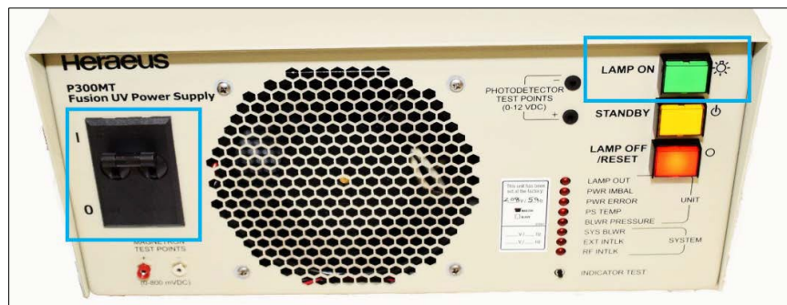
Figure 8: Lamp Power and Control Switch
